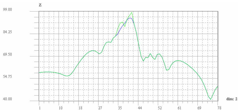
Figure 24 - Flight noise event for SPL at 1/3-octave band 1600 Hz (calculations) at measurement point No A2: blue line - SPL without impact of the ray reflected by wing; green line - SPL with impact of the ray reflected by wing
